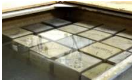
Fig No: 4.2 Curing of concrete cubs in water
